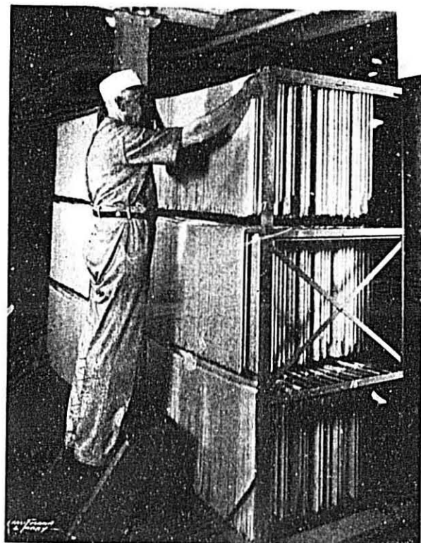
(Courtesy of National Macaroni Manufacturers Association) Fig. 13. Drying macaroni on sticks in drying room.
